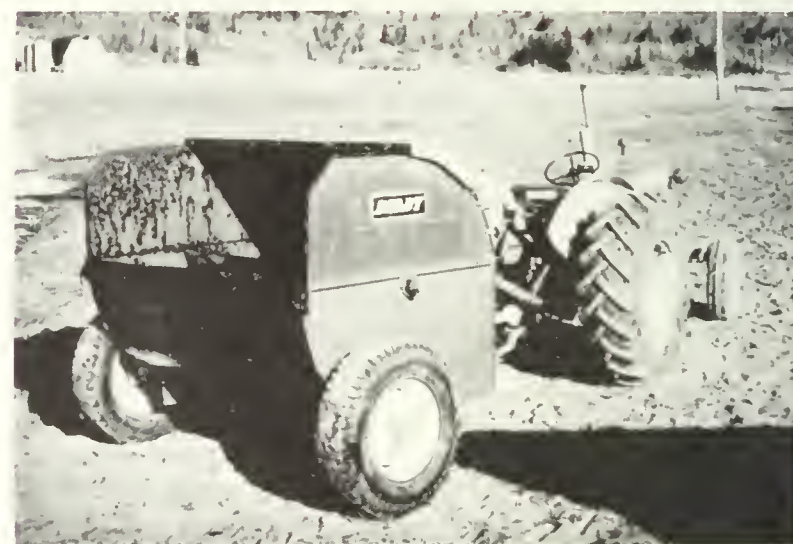
Figure 3.5.40 Rear discharge, chain-flail, tank-type spreader (courtesy Engineering Division, B.C. Ministry of Agriculture)
